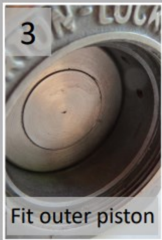
Method of pushing pistons past the seals
