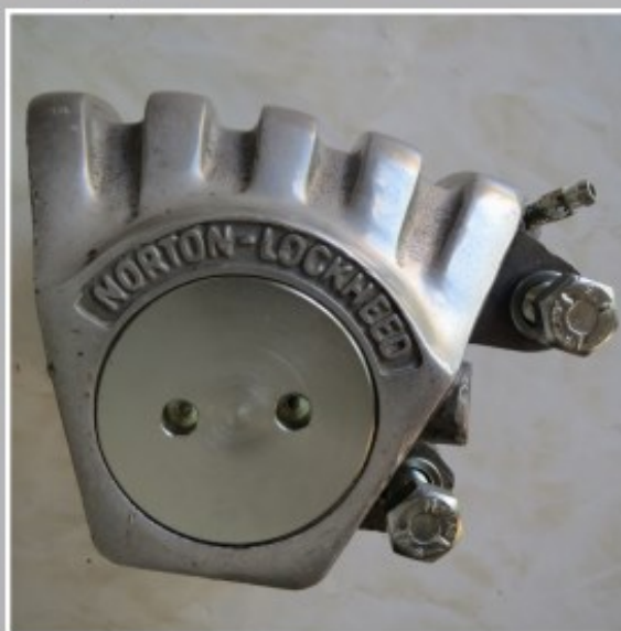
Fit caliper plug seal
